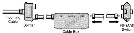
4 Connect a coaxial cable between the other OUT terminal of the Cable box and the A-IN terminal of the RF (A/B) switch.
