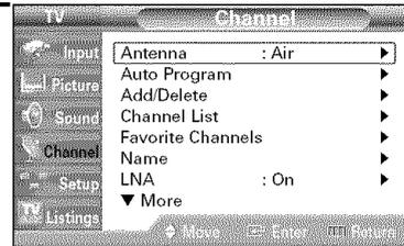
2 Press the ▲ or ▼ button to select "LNA", then press the ENTER button.
