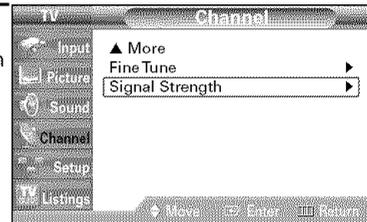
If the signal strength meter indicates that the signal is weak, physically adjust your antenna to increase the signal strength. Continue to adjust the antenna until you find the best position with the strongest signal.
