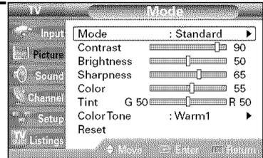
3 Press the ENTER button. Press the ▲ or ▼ button to select the desired picture mode (Dynamic, Standard, Cinema), then press the ENTER button.
