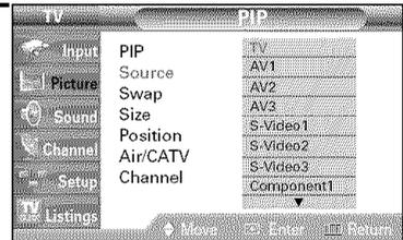
Press the ▲ or ▼ button to select an external signal, then press the ENTER button.
