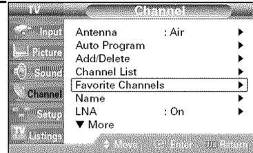
2 Press the ▲ or ▼ button to select "Favorite Channels", then press the ENTER button. Press the ▲ or ▼ button to select a channel, then press the ENTER button and a check mark will appear. Press the ENTER button again to deselect the selected channel and the check mark will disappear.
