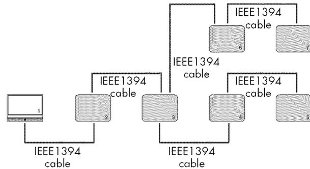
Do not connect D-Net (IEEE1394) Compatible devices in a way that creates a loop.
