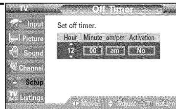
To activate Off Timer with the setting entered, set Activation to "Yes" by pressing ▲ or ▼ button.
