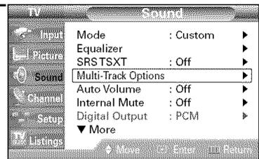
3 Press the ▲ or ▼ button to select "Multi-Track Sound", then press the ENTER button.
