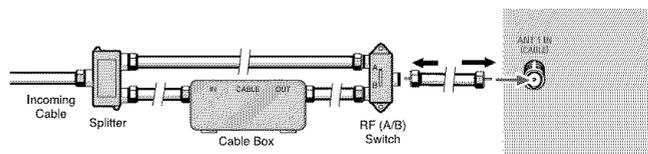
After you've made this connection, set the A/B switch to the "A" position for normal viewing. Set the A/B switch to the "B" position to view scrambled channels. (When you set the A/B switch to "B", you will need to tune your Set-Top Box to the Cable box's output channel, which is usually channel 3 or 4.)
