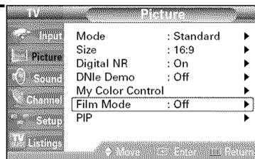
3 Press the ▲ or ▼ button to select "Off" or "On", then press the ENTER button.
