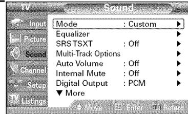
2 Press the ▲ or ▼ button to select "Digital Output", then press the ENTER button.
