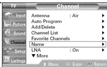
3 Press the  $\blacktriangle$  or  $\blacktriangledown$  button to move to the channel to be assigned to a new name, then press the ENTER button. Press the  $\blacktriangle$  or  $\blacktriangledown$  button to select a letter, a number or a blank. (Results in this sequence: A...Z, 0...9, +, -, \*, /, blank).
