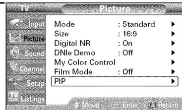
3 Press the ENTER button to select "PIP". Press the ▲ or ▼ button to select "On", then press the ENTER button. The sub picture appears in the corner of the screen.
