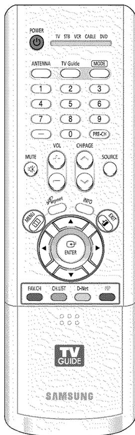
1 Press the MENU button. Press the ▲ or ▼ button to select "Channel", then press the ENTER button.
