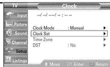
5 Press the ◀ or ▶ button to move to "Month", "Day", "Year", "Hour", "Minute", or "am/pm". Set the clock you want by pressing the ▲ or ▼ button, then press the ENTER button.
