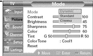
4 Press the ▲ or ▼ button to select a particular option (Contrast, Brightness, Sharpness, Color, or Tint), then press the ENTER button.
