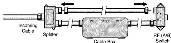
5 Connect the last coaxial cable between the OUT terminal of the RF (A/B) switch and the ANT 1 IN (CABLE) on the TV.
