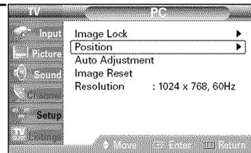
5 Adjust the position of picture by pressing the ▲/▼/◀/▶ button.
