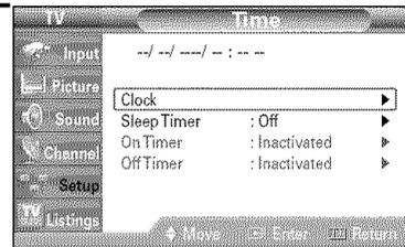
3 Press the ENTER button to select "Clock Mode". Press the ▲ or ▼ button to select "Manual", then press the ENTER button.
